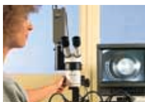
In the stereoscope inspection, parts from ongoing production are continually monitored and documented.
