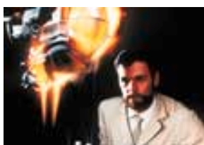
In quality assurance tests products are treated rougher than in the field – here a flame test for full face masks.
