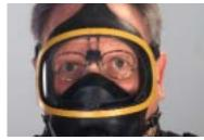
For use by workers who must wear corrective lenses, the spectacle kit can be easily inserted into the facepiece. The kit includes a wire support, rubber guide and one pair of metal-frame spectacles.
