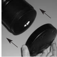
motion for attaching spark cover
