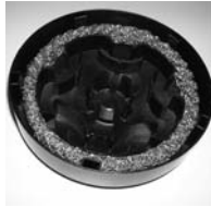
check for optional spark arresting material
