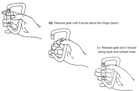
Gate should rotate 90 degrees and engage nose (lock).
