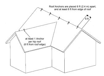
Roof framing to which the Roof Anchors are attached must be strong enough to support the required loads. Roof members should be free of cracks, splits, knots, rot or deterioration which may weaken the framing. <u>Do not</u> install Roof Anchors on unsupported roof structures such as eaves or gable overhangs. <u>Do not</u> install Roof Anchors on fascia boards.
