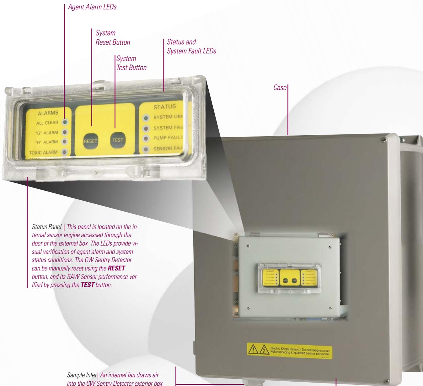
**Status Panel** | This panel is located on the internal sensor engine accessed through the door of the external box. The LEDs provide visual verification of agent alarm and system status conditions. The CW Sentry Detector can be manually reset using the **RESET** button, and its SAW Sensor performance verified by pressing the **TEST** button.
