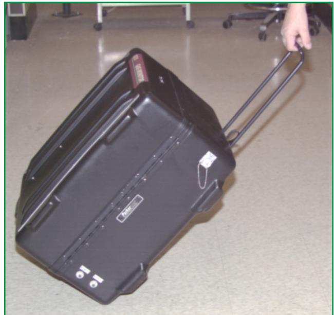
Transportable Chillgard RT Monitor with built-in handle, ready to transport.
