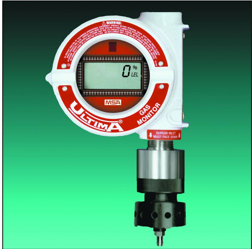
**C**ontinuous lower explosive limit (LEL) gas detectors must operate in a variety of ambient conditions. IR technology is immune to the poisoning effects of certain compounds and is not affected by oxygen-deficient conditions. The Ultima IR Gas Monitor will operate unattended for long periods of time without maintenance in ever-changing environmental conditions. The Ultima IR Gas Monitor is designed for extended, trouble-free operation, with minimal zero drift over the rated temperature range.
