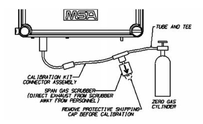
Figure 4-5. Using Zero Gas Cylinder for Zero Calibration
