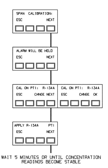
Figure 3-4a. Span Calibration
