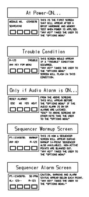
Figure 3-2a. Start-up and Normal Operation Screens
