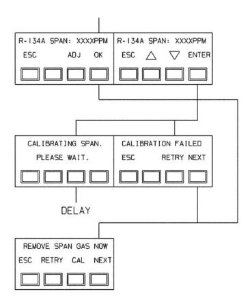
Figure 3-4b. Span Calibration Continued
