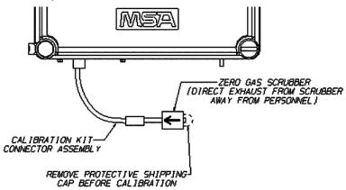
Figure 4-4. Using Zero Scrubber for Zero Calibration
