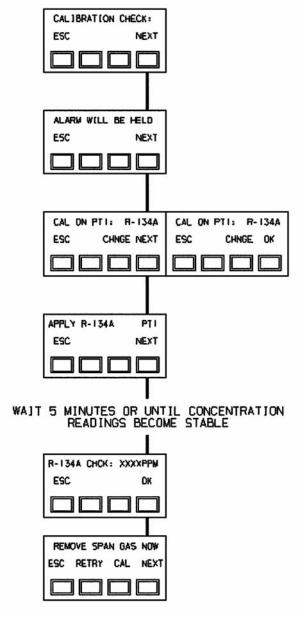
Figure 3-6. Check Calibration
