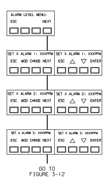
Figure 3-11. Alarm Level Screen
