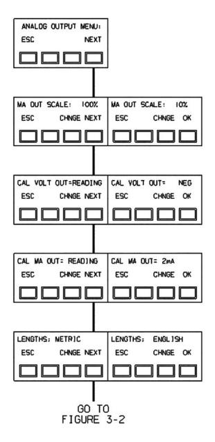
Figure 3-15. Analog Output Screen
