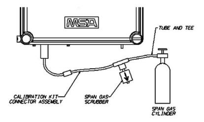
Figure 4-6. Span Calibration
