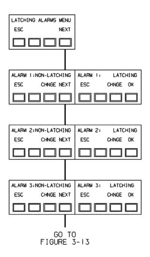
Figure 3-12. Alarm Latching Screen
