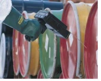
The Passport PID II Organic Vapor Monitor is a convenient, portable instrument for detecting low concentrations of volatile organic compounds (VOCs). The Passport PID II Monitor's compact design supports a variety of monitoring applications:
