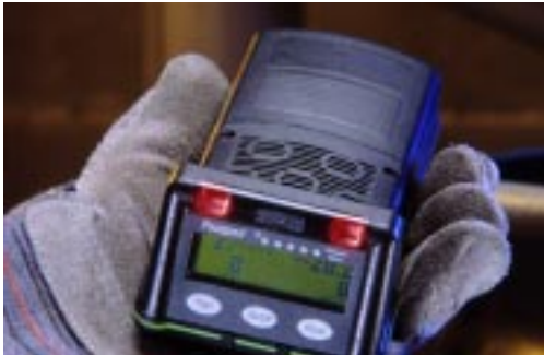
Figure 8 Typical, Compact Portable Gas Detector
