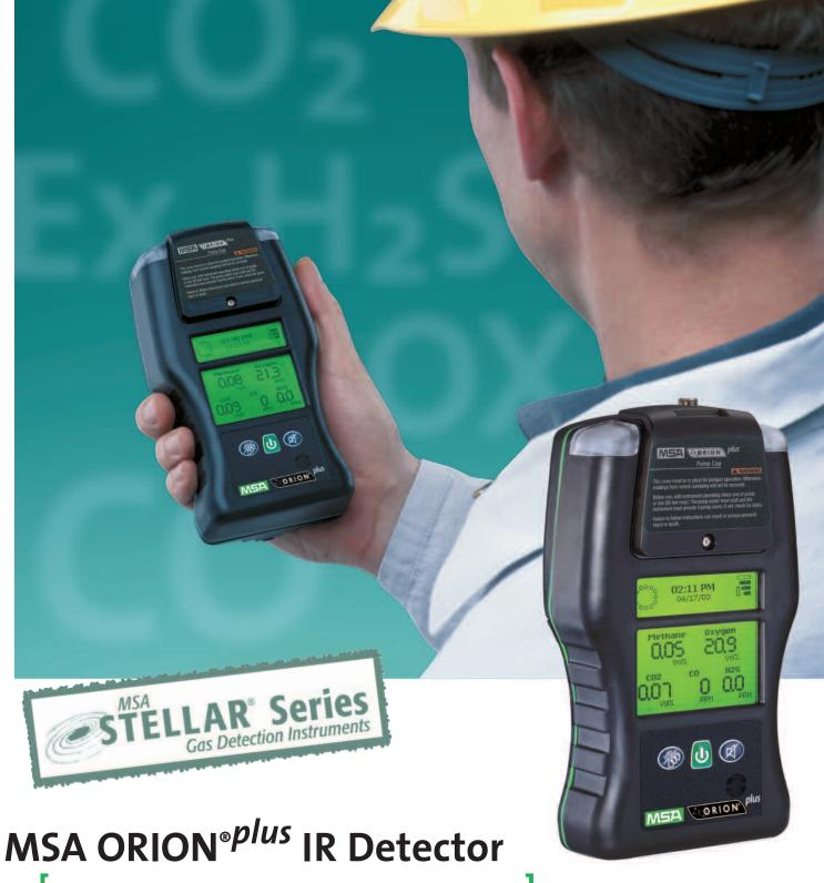
Versatile and rugged; five gases with infrared
