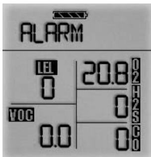
Figure 3-4b. Pump Alarm on the Display
