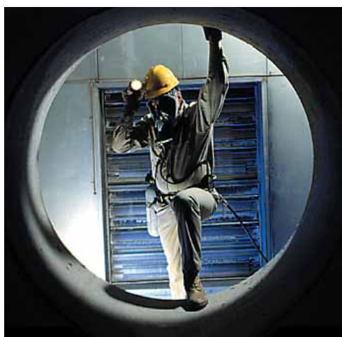
Escape-cylinder option used in confined space application.
