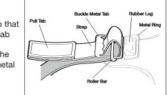
**Note:** It is important to have the folded side of the elastic strap face up, so the strap will lay flush against the head when it is pulled tight.
