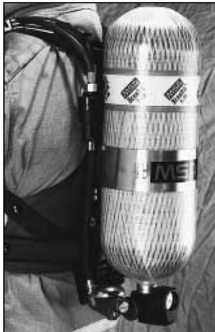
*MMR First-stage Regulator is mounted to cylinder backplate.*
