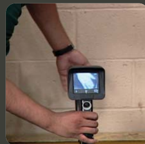
The TIC still functions after drop
