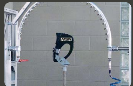
IPX4 tests resistance against heavy rain
