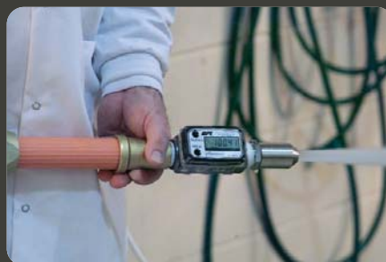
Nozzle used for IPX6 Test
