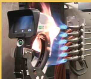
NFPA 1981-2002 Edition simulated for Direct Flame/ Heat Exposure
