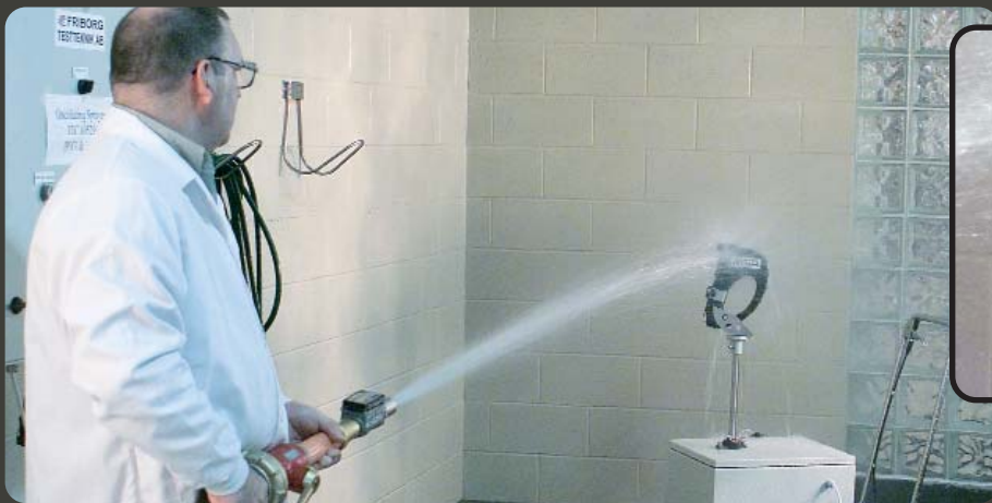
IPX6 Water Ingress Test against stronger jet spray
