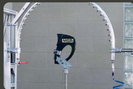
IPX4 tests resistance against heavy rain
