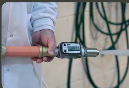
Nozzle used for IPX6 Test
