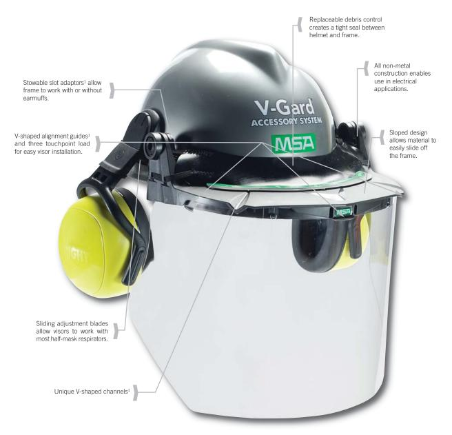
V-Gard Frame for Slotted MSA Caps, with debris control (PN 10115730). Shown with V-Gard clear molded, propionate visor (PN 10115855) and MSA left/RIGHT<sup>®</sup> (HIGH) earmuffs (PN 10087422).
