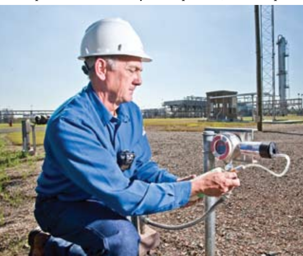
Fig. 1. Technician calibrating MSA ULTIMA X detector
