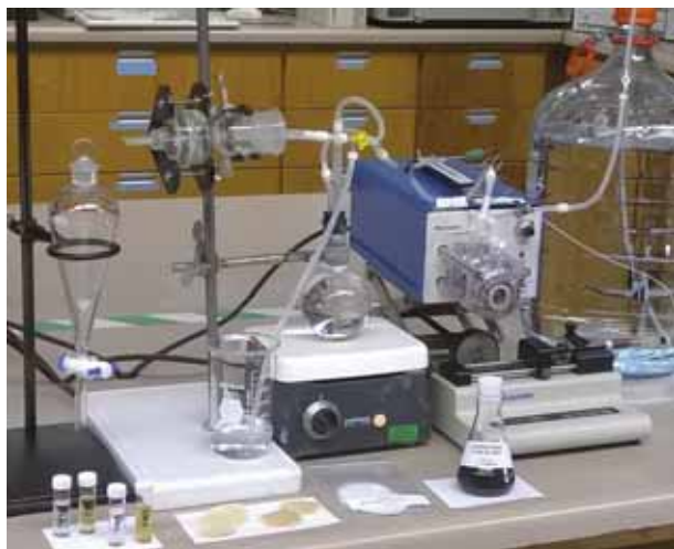
Figure 1. Laboratory apparatus used for chromatography analysis to determine oil separation efficiency by nylon spunbond fabric.
