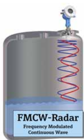
Figure 1. FMCW radar sends a continuous wave that reflects off the surface and returns to the antenna. The shift in frequency determines the level in the tank.
