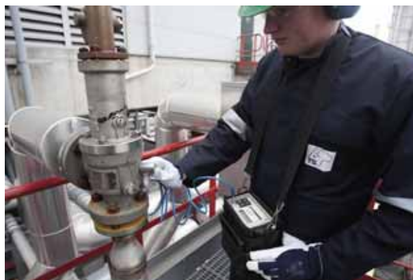
Figure 6. Ultrasound measurement of internal leakage safety valve.
