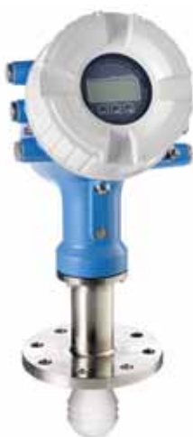
Figure 3. An 80 GHz radar instrument, such as this Endress+Hauser Micropilot NMR81, provides 0.5 mm accuracy, can be mounted closer to the tank wall, and its antenna requires only a small hole in the tank roof of 2 – 4 in.
