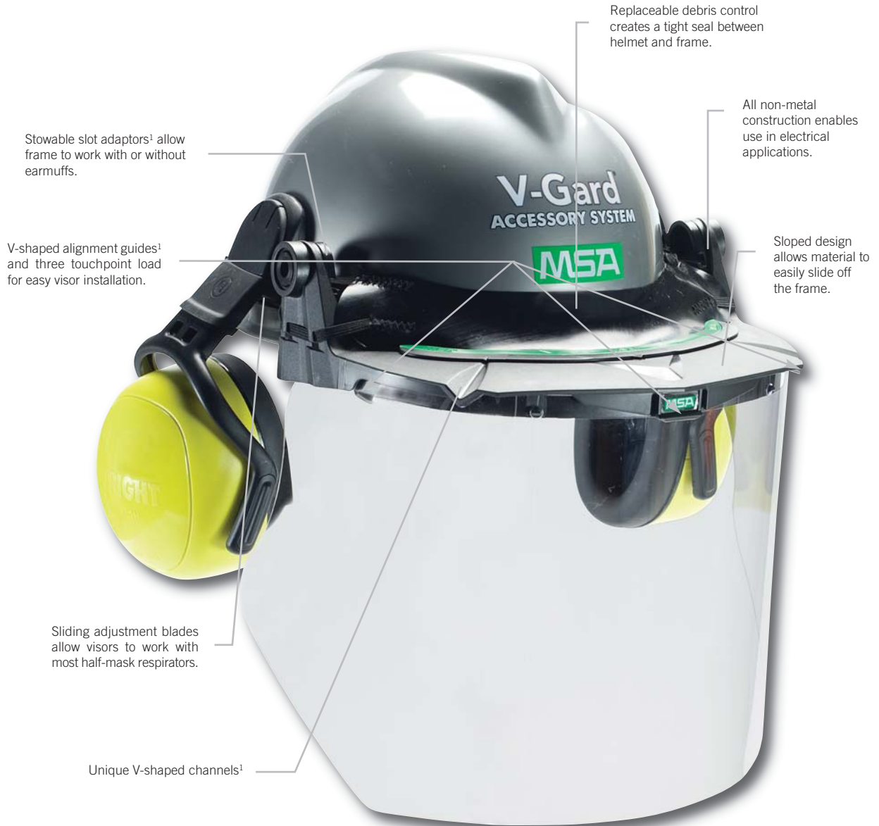
V-Gard Frame for Slotted Caps, with debris control. Shown with V-Gard clear molded, polycarbonate visor and MSA left/RIGHT® (HIGH) earmuffs.
