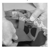
5. Use a large screwdriver and pliers to unscrew the two (1/2 inch long) front chinstrap retention screws.
