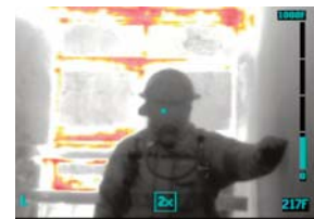
Same picture with 2X Digital Zoom activated showing low-sense imagery on the display of an E5200HD 2 TIC
