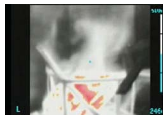
Low Sense image detail with Heat Seeker enhancing the heat source with red isotherm
